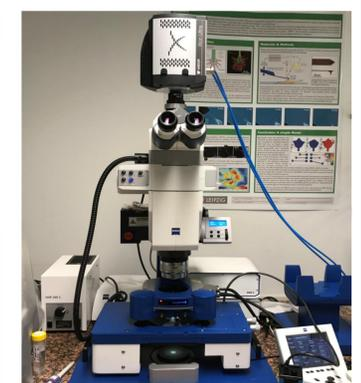
JPK HybridStage™ on a Zeiss upright AxioZoom V.16 fluorescence microscope with an Andor EMCCD camera for force mapping experiments on non-transparent tissue samples. Image courtesy of Josef Käs and Thomas Fuhs, Uni Leipzig, Germany.
