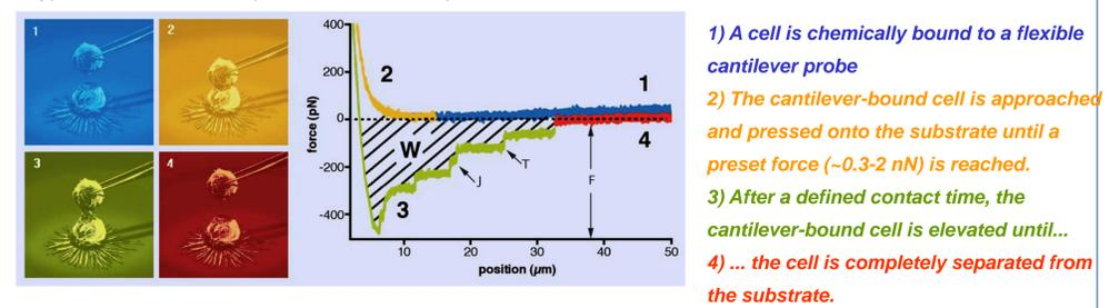
The flexible cantilever bends upwards/downwards as the cell is pressed towards/ separated from the surface. The cantilever probe can be thought of a spring which allows for converting the deformation into units of force. Consequently, adhesive interactions, such as maximum adhesion and single unbinding events can be quantified in the single cell range (pN-nN). Attachment can be done by functionalization or aspiration (FluidFM).
