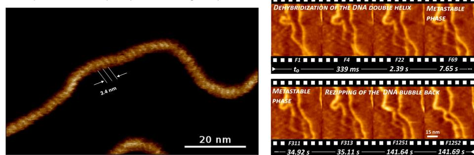
Application of high-speed AFM for studying the pUC19 DNA double helix (left), showing the double helical repeat of 3.4 nm
